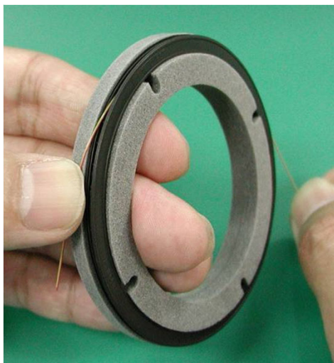
Reeling of fiber using a hand spooling jig, "Spool Holder"
