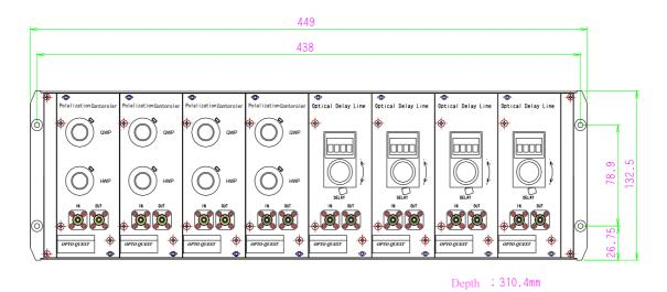
Combination example: RDLA (4ch) + Polarization Controller RPCA (4ch) \*The Wavelength Tunable Filter Unit and Variable Optical Attenuator Unit can also be combined.
