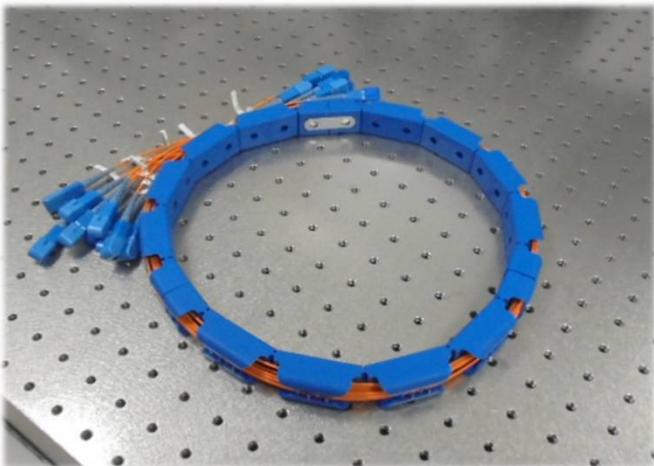
Storing the fiber patch cords in a compact circle
